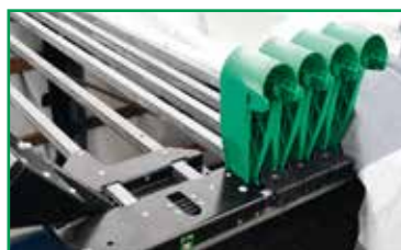
Komplette planenschonende Faltung Full tarpaulin-protecting folding
